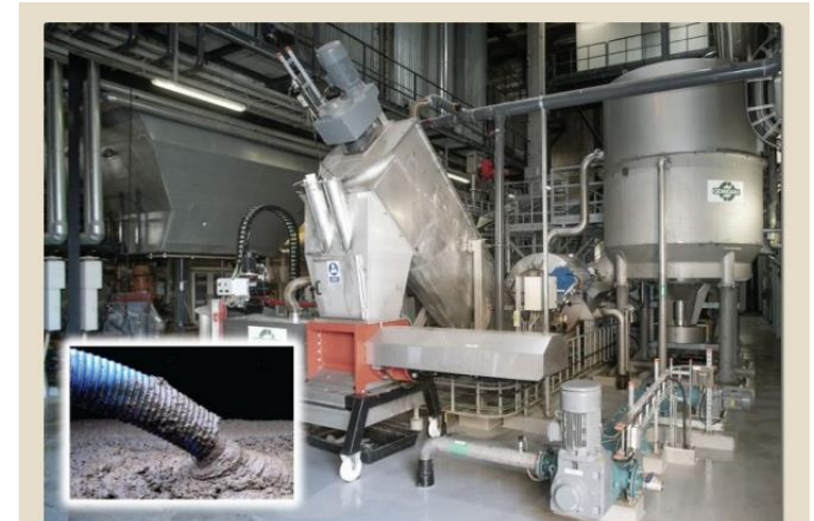
The food waste pretreatment plant manufactured by Gemidan Ecogi at AffaldPlus processes 27,500 tons/year of packaged food. The output is a biopulp (inset) with solids content of about 17%.
