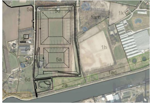
Pit heat storage (700.000 m 3 – 1.000.000 m 3 ), 150 MW
