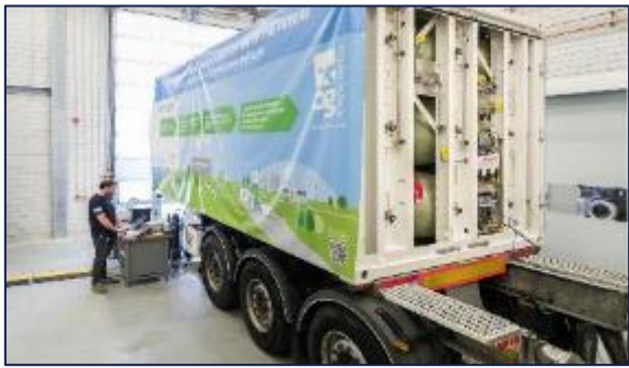
Hydrogen tube trailer – ready for operation test
